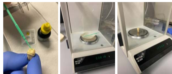
Left: application of primer in tooth cavity Middle: weight of applicator with remaining primer Right: weight of cavity with primer
